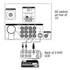
The S-Video connection on the rear of the TV is used for the playback of S-VHS VCR tapes, Video Discs, Video Games or Compact Disc-Interactive (cd-i) discs. Better picture detail and clarity is possible with the S-Video playback as compared to the picture from a normal antenna (RF) connection.
